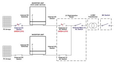
• Open the external DC disconnect switch (blue in previous picture) outside the inverter (IEC 60364-7-712.536.2.2)
