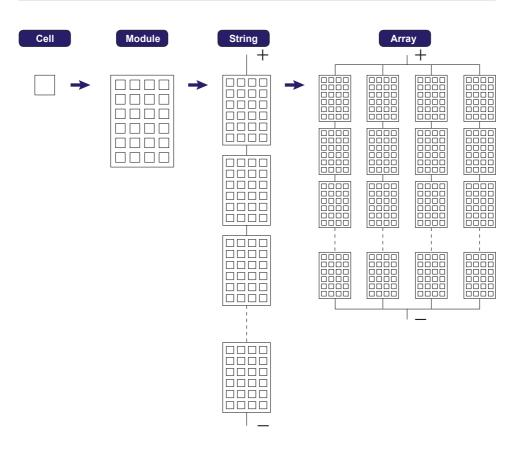
A ATTENTION - The current of each array must fall within the rating value limits of the inverter (see "Technical data").
