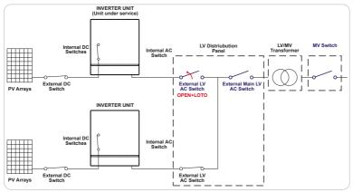
• Open the external AC disconnect switch or the main external AC disconnect switch (blue in previous picture) outside the inverter (IEC 60364-7-712.536.2.2). In case none of the LV AC switches are present, the MV switch must be opened.
