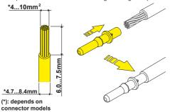
Insert the crimped terminal contact into the insulator body of the connector, until you hear the click indicating that the terminal is engaged inside the connector.
