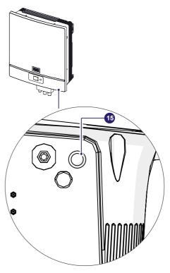
This physical button allows to enable WiFi access point.
