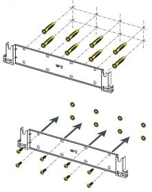
· Attach the bracket (05) to the support.
