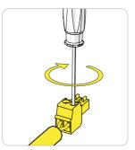
•Connect the wired screw terminal block to the Digital Input connector (12).
