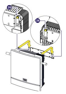
Remove the handles (25) or eyebolts and tighten the supplied two side bracket screws (18) (see paragraph "3.5.2 Tightening torques") to avoid the tilting of the bottom part of the inverter.
