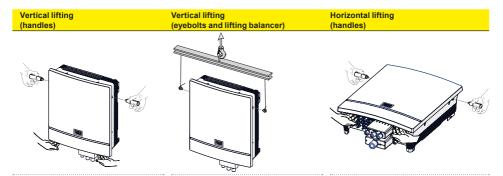
ATTENTION - DO NOT grab the equipment from the rear flange! Risk of injury due to cutting surfaces and risk of equipment damage. Always use proper lifting equipment!
