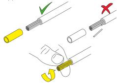
· Crimp the terminal to the conductor using the designated pliers.
