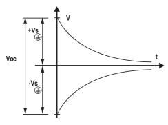
NOTE – The internal resistance of the voltmeter tends to zero the voltage present on the PV generator due to the capacitive effect. 8.6.2 Behaviour of a system with leakage
