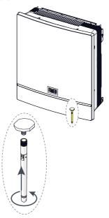
•A padlock can be installed to lock the inverter to the bracket so that it cannot be disassembled by outsiders.
