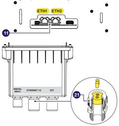
${\mathbb A}$  ATTENTION – If the inverters need to be connected in daisy chain or ring configuration use both connectors.
