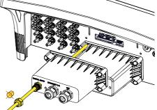
• Install the 2 poles screw terminal block (supplied) on the cable (see paragraph "3.5.2 Tightening torques").
