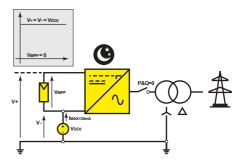
Array terminal voltages with respect to ground during night-time PID recovery operation (inverter is off-line).
