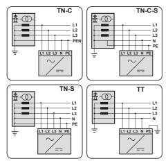
NOTE – The connection of the neutral (N) on the inverter is optional (dashed line on the above schematics); the inverter will automatically detect the presence or absence of the connection without any setting by the user.
