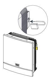
Remove the protective cover from the connector of the Wi-Fi antenna located on the bottom side of the inverter. Install the Wi-Fi antenna by screwing it into the specific connector (14).
